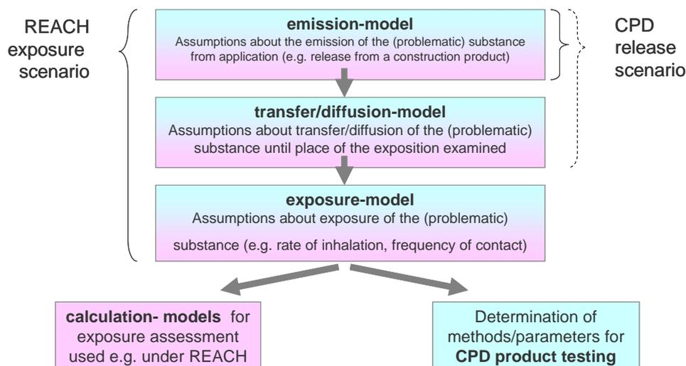
Figure 3: Comparison between exposure scenario and release scenario
